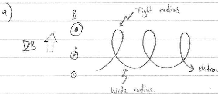
Gradient in B field strength  $\perp$  to  $\underline{B}$
